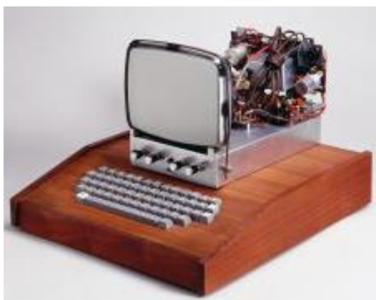
Fig. 8. The Apple I computer, devised by Steve Wozniak, Steven Jobs and Ron Wayne, was a basic circuit board to which enthusiasts would add display units and keyboards ( Source: History of computers )
