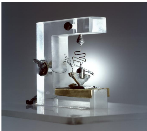
Fig. 2. The first transistor, developed by Walter Brattain and John Bardeen called "point contact transistor" (Source: Nokia USA Inc. and AT&T Archives)
